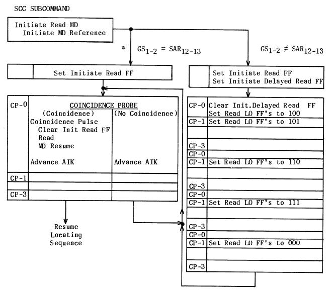
\* It should be noted that even though  ${\rm GS}_{1-2}={\rm SAR}_{12-13}$ , if a read operation follows a write operation before approximately 40 usec have elapsed, all or a portion of the Read LO FF counting delay  $({\rm GS}_{1-2} \neq {\rm SAR}_{12-13})$  will be carried out until each Read LO FF is in its "0" state.
